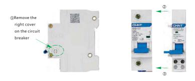
After OUVT-X3 is assembled with the circuit breaker, mount them to TH35-7.5 steel mounting rail.
